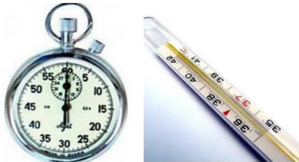
Figure 1.5. Stopwatch, thermometer - examples of interval scale
